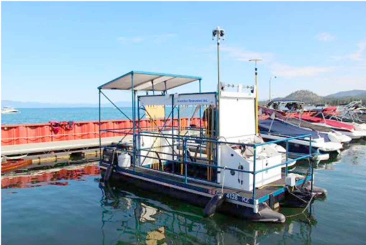
Figure 1. This boat built by Inventive Resources has a panel of UV lights that is lowered to expose aquatic invasive plants to UV light.
