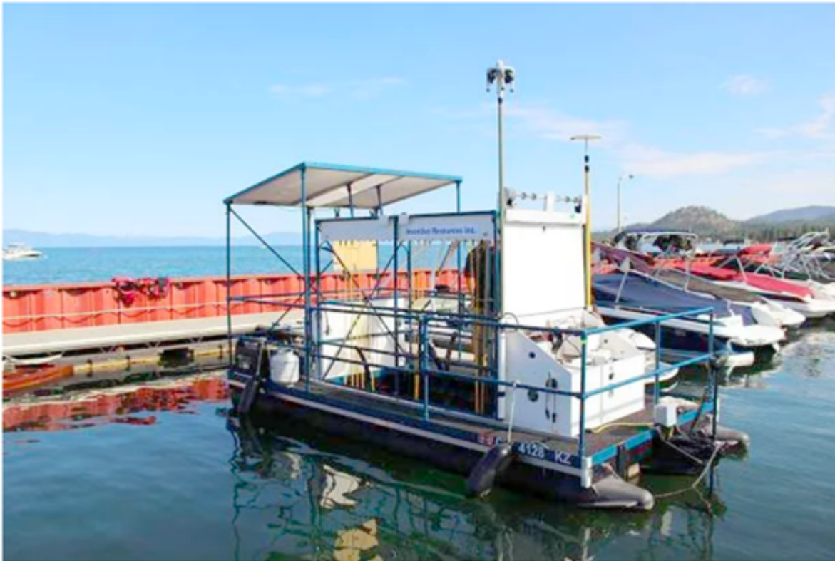
Figure C-13. This boat built by Inventive Resources has a panel of UV lights that is lowered to expose aquatic invasive plants to UV light.
