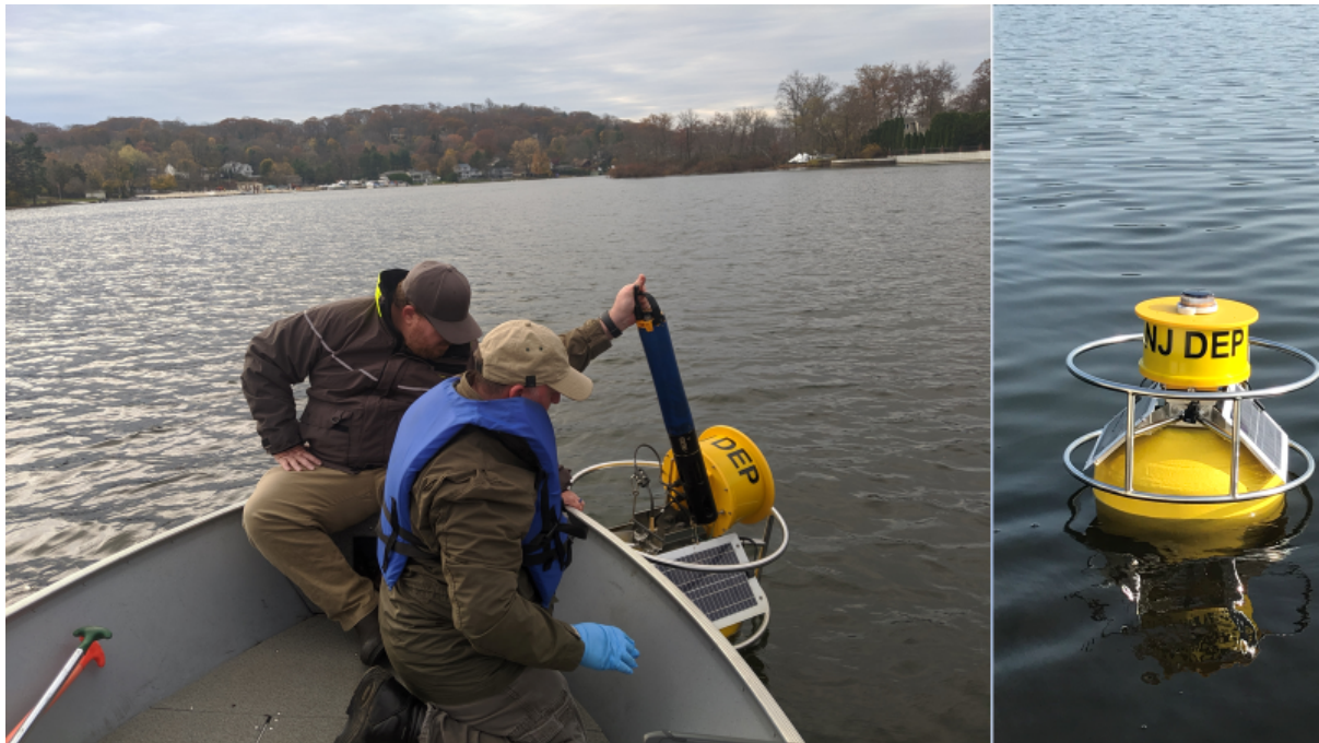
Figure 4-14. High-frequency monitoring buoy deployed at Lake Hopatcong, NJ.
