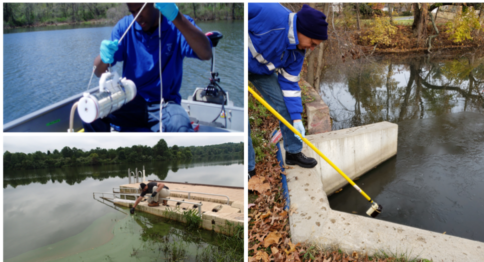
Figure 4-9. Examples of several ways to collect grab samples for cyanobacteria.
