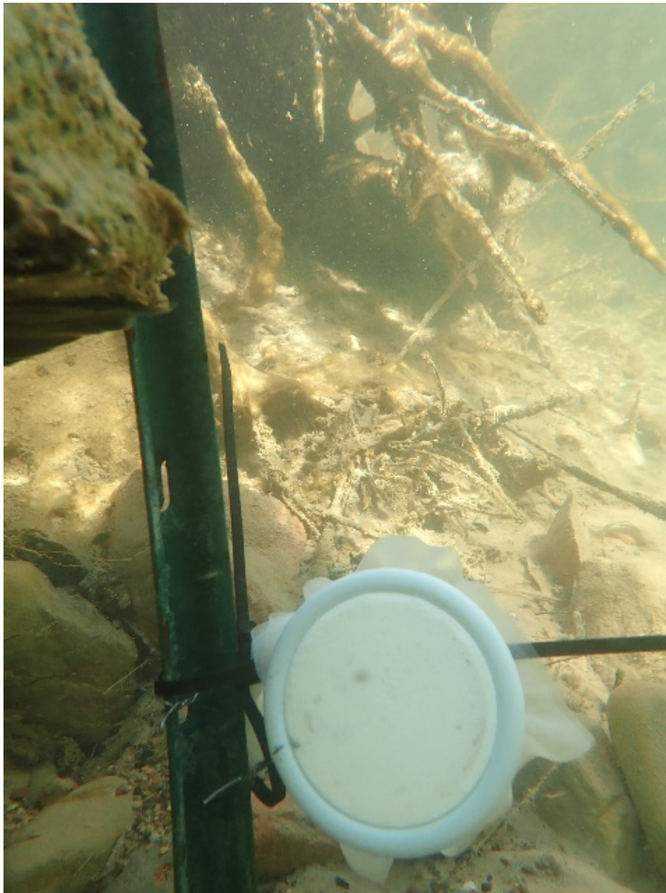
Figure 4-12. Deployment of 2.5-inch SPATT sampler in the North Fork Virgin River, Zion National Park, to evaluate cyanotoxins associated with a benthic mat.
