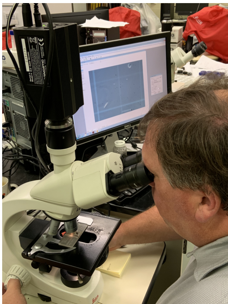
Figure 4-6. Using a microscope to identify cyanobacteria.
