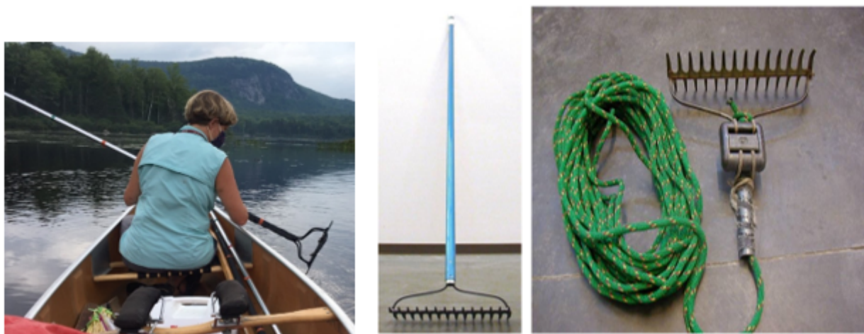
Figure 4-11. Rake sampling can be used for benthic cyanobacteria.
