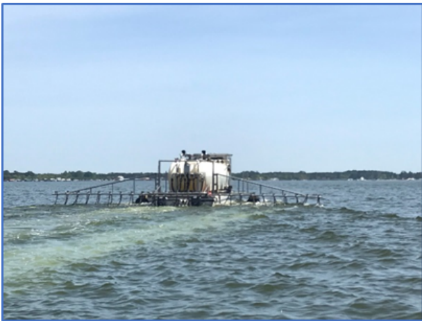
Figure C-10. Applying P-binding compounds to a lake.
